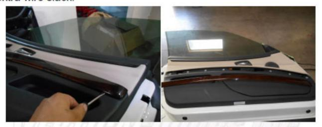
Remove all the wire clips from the front of the door to gain the extra wire slack needed. You will have to cut and extend 2 cables for one of the door sensors as shown below.
